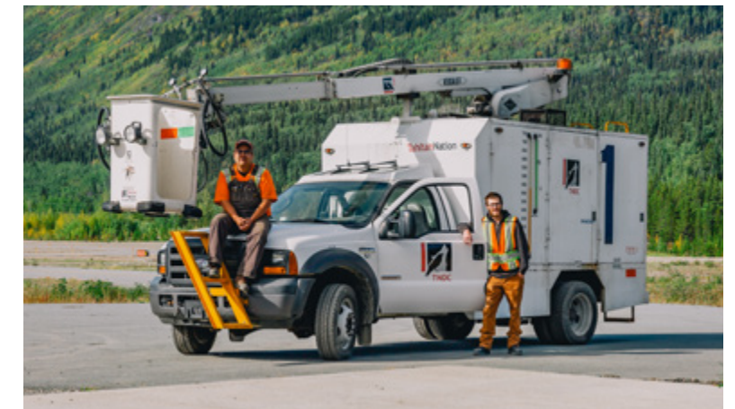
Above: Grant Louie and Tyson Fletcher from TNDC's Airport services team on our De-ice unit, used to spray de-ice fluid on the aircrafts.
